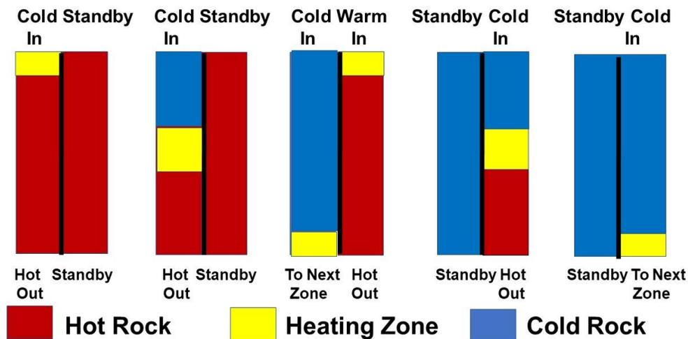
Fig. 4. Sequential Heat Recovery from Two Crushed Rock Zones (Nominal height 20 m and width 25m)
