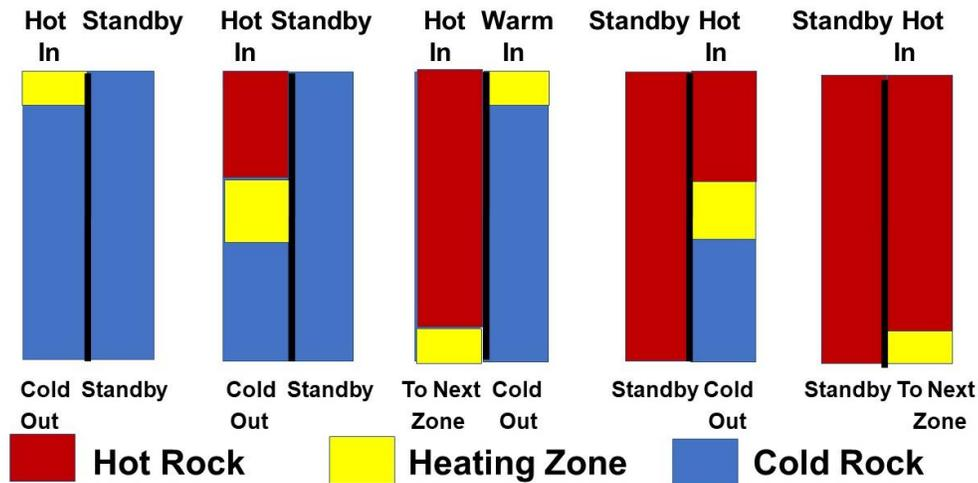
Fig. 3. Sequential Heating of Two Crushed Rock Zones (Nominal height 20 m and width 25m)
